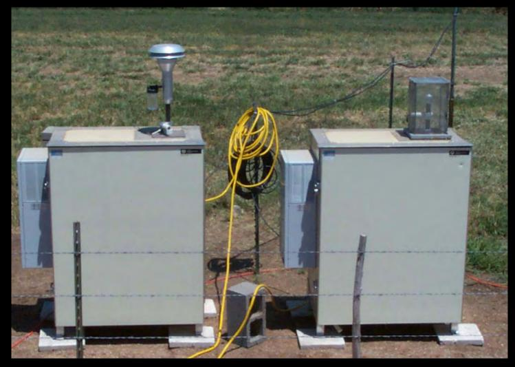
Tapered-Element Oscillating Microbalance (TEOM)
