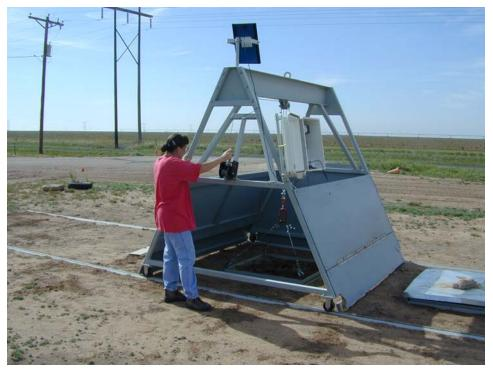
Figure 3. A lysimeter being weighed using a single, S-type load cell suspended from the rolling crane. Three sides of the crane were enclosed to deflect the prevailing southwesterly winds and to minimize eddy currents.
