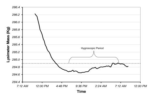
Figure 7. A typical daily plot of lysimeter mass. The hygroscopic period of the lysimeter manure is evident in the evening and early morning hours.
