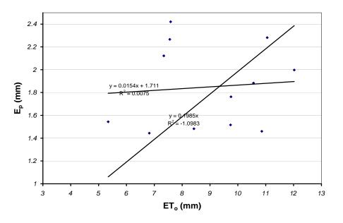
Figure 6. Data from the Phase II configuration reveals that  $E_p$  and  $ET_o$  are poorly correlated. Forcing the regression through the origin suggests that  $E_p$  is about 20% of  $ET_o$  but degrades the fit of the linear model.
