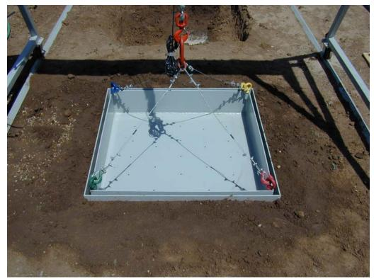
Figure 1. View of an empty lysimeter pan mounted inside the retaining pan. Drainage holes are visible in the bottom of the pan. In the original configuration, wire slings attached to the corners of the pan were gathered to a common link and suspended from an S-type, overhead load cell on an A-frame superstructure visible in the upper left and upper right corners of the photo.
