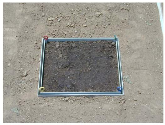
Figure 2. A view of a lysimeter pan packed with a Sherm silty clay loam and topped with unprocessed feedyard manure.
