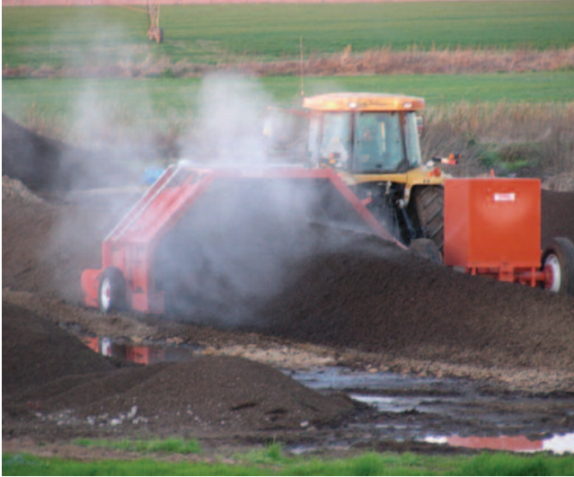
A tow-behind compost turner runs through a steaming windrow of dairy manure in California's Central Valley.
