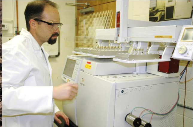
Figure 2. GHG samples being analyzed on Varian 450 gas chromatograph
