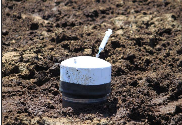
Figure 1. NFT-NSS chamber deployed on manure pack at open-lot dairy
