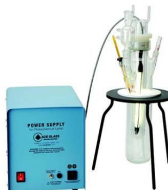
Figure 4: Photoreactor where the experiments will be carried out.
