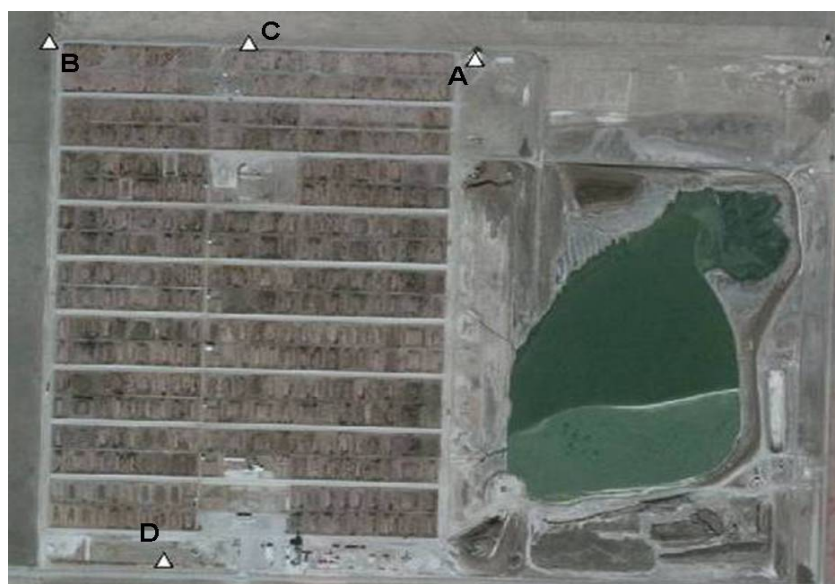
Figure 1. Overhead photograph of the cooperating feedyard. Instruments were deployed so that we could measure PM_{10} and TSP mass concentration and atmospheric extinction simultaneously measured along the downwind boundary of the feedyard. Transmitter is at A; receiver (photometer) is at B; upwind TEOM is at D; and downwind TEOMs are at C.
