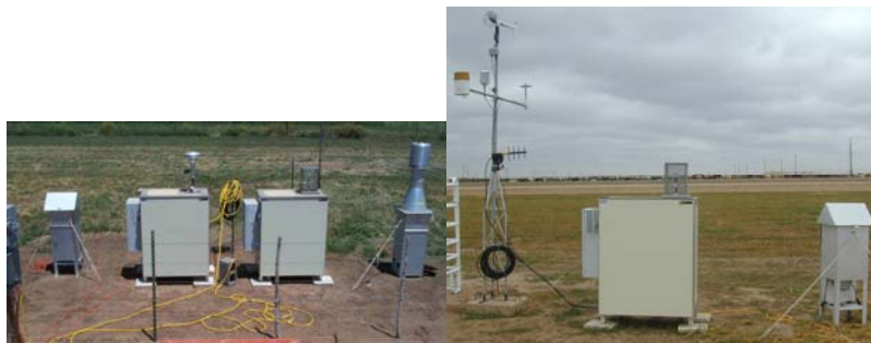
Figure 3. Downwind samplers at location C (left). From left are a federal reference method, high-volume TSP sampler; a TEOM configured for PM 10 ; a TEOM configured for TSP; and a federal reference method, high-volume PM 10 sampler. (Right) Upwind monitors at location D.
