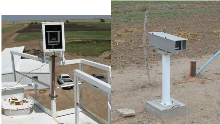
Figure 2. (a) Looking E at the transmitter shelter atop a large water tank at location A (left). (b) Looking NW at the pedestal-mounted photometer/receiver at location B (right).
