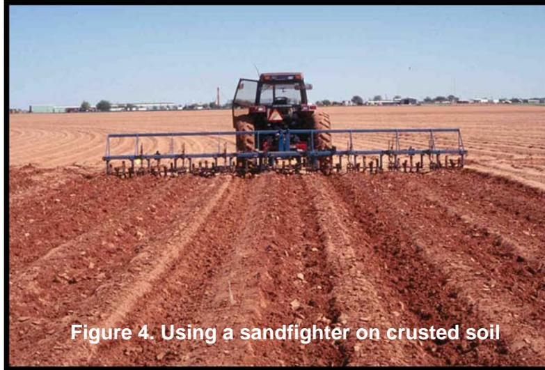
Figure 4. Using a sandfighter on crusted soil
